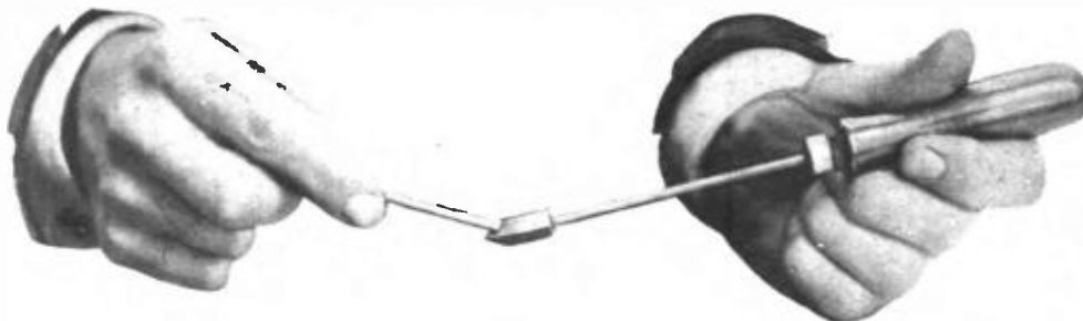
Get the iron hot and then tin it with the solder
